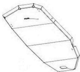
Fuel tank protection
