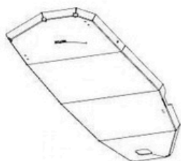
Fuel tank protection
